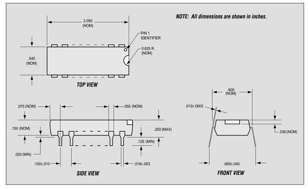
Figure 13. Mechanical Data 40-Pin Plastic DIP
