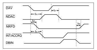
Figure 9. Acceptor Handshake Timing
