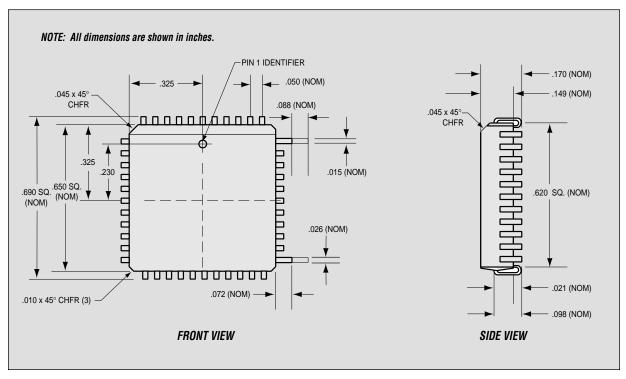
Figure 14. Mechanical Data 44-Pin PLCC
