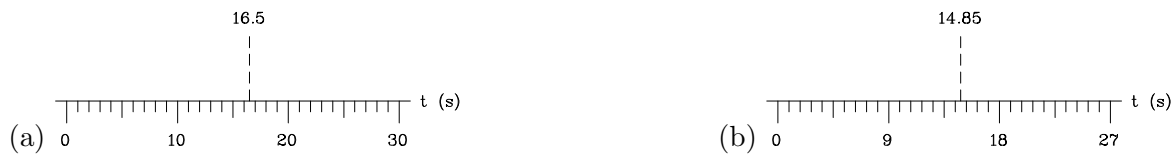
Figure B.1: (a) 1 mm (on paper) : 1 s; (b) 1 mm (on paper) : 0.9 s
