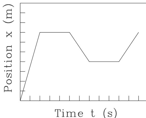
2. By applying a slight push to the air car, generate a trace of constant velocity. Make sure the air track is level first! Each student should generate their own trace, save it as a file. Then using PHYSICA they should determine the actual velocity (slope of  $x$  vs.  $t$ ) from their graph.
