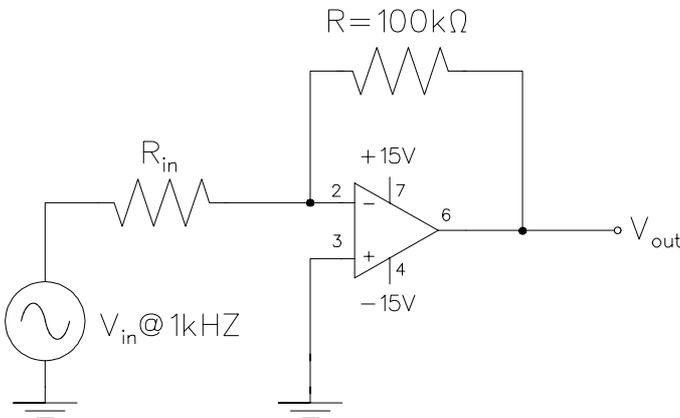
Figure 12.2: An inverting amplifier
