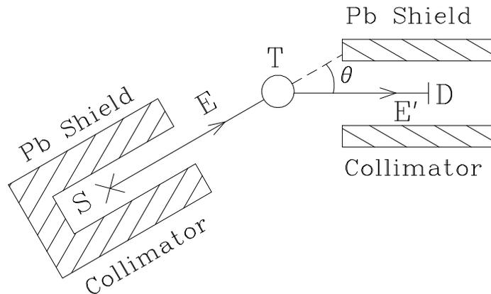
Figure 7.1: Compton scattering arrangement
