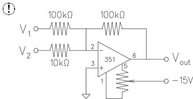
Wire up a summing amplifier, as shown. Use the  $\pm 10\text{V}$  supply as  $V_1$  and the  $\pm 1\text{V}$  supply as  $V_2$ . Measure  $V_{\text{out}}$  for six or more combinations of input voltage values. Keep one value constant for at least three values of the other and *vice versa*.
