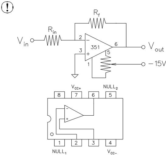
Wire the circuit shown with  $R_f = 100\text{ k}\Omega$  and  $R_{in} = 10\text{ k}\Omega$  (gain  $\approx 10$ ); connect input to common, and adjust the balance potentiometer until the op-amp output is nearly zero ( $\leq 1\text{mV}$ ). Set DMM to an appropriate scale.
