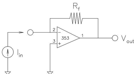
Wire up the current-to-voltage converter circuit (note that this corresponds to simply interchanging the input and ground connections in the circuit of Section 2.3). Here we emphasize the fact that the input is explicitly a current, while the output is a voltage:
