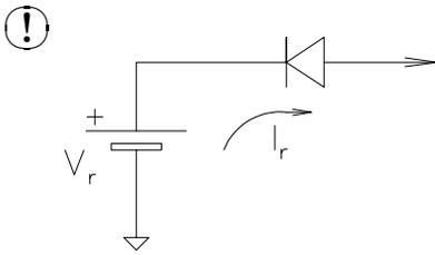
Using a signal diode 1N914, wire the following input circuit to measure the reverse bias current of the diode. Select the value of  $R_f$  necessary to give a reasonable  $V_{out}$ . Use reverse bias voltages  $V_r = 1, 2, \text{ and } 5\text{V}$ .
