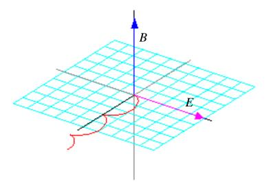
Another interesting case occurs when the initial velocity is zero and the electric field is perpendicular to the magnetic field. Let's say that
