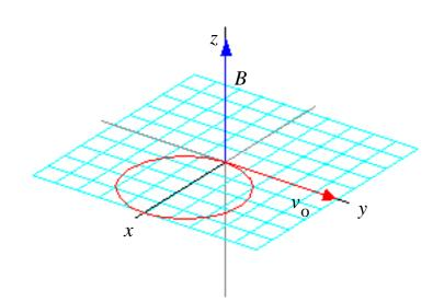
If, in addition, the initial velocity has a component parallel to the magnetic field, the path is a spiral, or *helix*.
