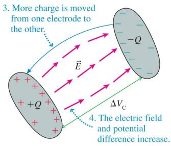
The charge  $\pm Q$  on each electrode is proportional to the potential difference  $\Delta V_{\mathbb{C}}$  between the electrodes:
