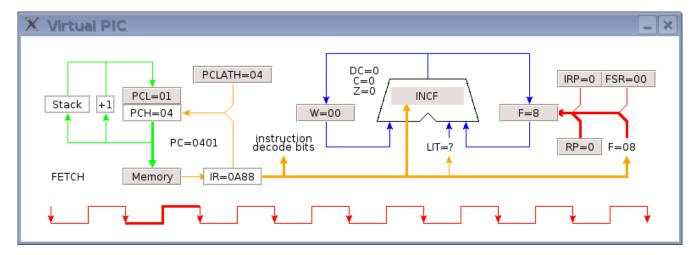
During clock cycle 2, the file register data at address 8 is being accessed. The PC begins to access the next instruction in program memory.
