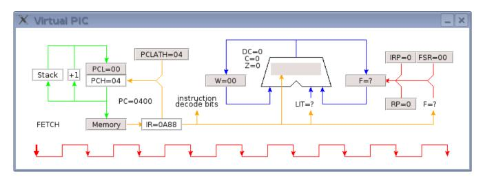
The binary representation of the 'incf PORTD' instruction (0x0A88) has been fetched from program memory location 0x0400 pointed to by the program counter (PC) and placed in the Instruction register (IR) on the falling edge of the PIC clock. In this case, the IR contains the 7-bit address of file register PORTD (8) as well as the code for the ALU operation that will be performed. The IR also specifies several decode bits that serve to control the internal operation of the PIC.
