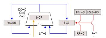
called W. The right input is connected to an array of 512 file registers. A memory address (path shown in red) selects which file register output will be connected to the ALU input. Alternately, a literal (constant) can be selected as the right input to the ALU. The output of the ALU is connected to both the W and file register inputs.
