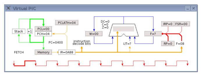
During the first clock cycle, the IR output is decoded as the file register address for PORTD (8), the ALU operation and the PIC hardware control bits. The program counter output is routed to an incrementing circuit. The file register read/write control is set to read.
