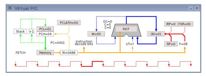
During clock cycle 4, the incremented data is presented to the file register. The file register read/write control is set to write. The program memory read cycle continues.
