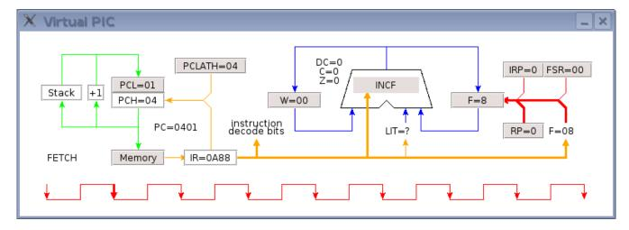
On the falling edge of clock cycle 1, the file register address for PORTD (8) has been decoded and is ready to use. The program counter is loaded with the output of the incrementing circuit, that is, the PC has been incremented and is now pointing to the next program memory location.
