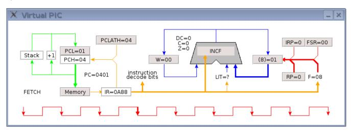
On the falling edge of clock cycle 3, the file register data has been incremented and is ready at the output of the ALU. The program memory read cycle continues.
