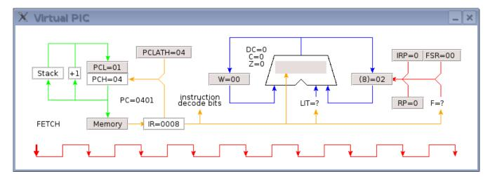
On the falling edge of clock cycle 4, the incremented data (02) is written to file register address 8. The instruction at memory location 0x0401 is written to the instruction register, terminating the current and beginning the next instruction cycle.
