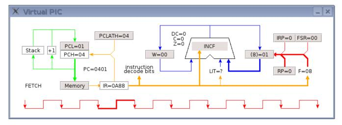
During clock cycle 3, the file register data is operated on by the ALU. The program memory read cycle continues.
