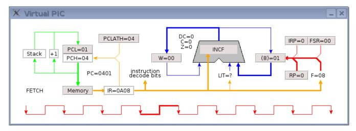
During clock cycle 4, the W register is selected as the destination for the ALU data.
