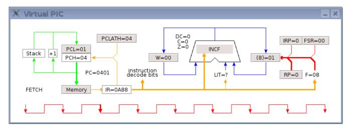
On the falling edge of clock cycle 2, the file register data (0x01) read at address 0x08 is ready to use. The program memory read cycle continues.
