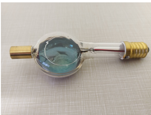
Figure 6.2: An LD Didactic photocell, type 558 77. The potassium coating on the back surface of the cell is the cathode, and the wire ring suspended above it is the anode.
