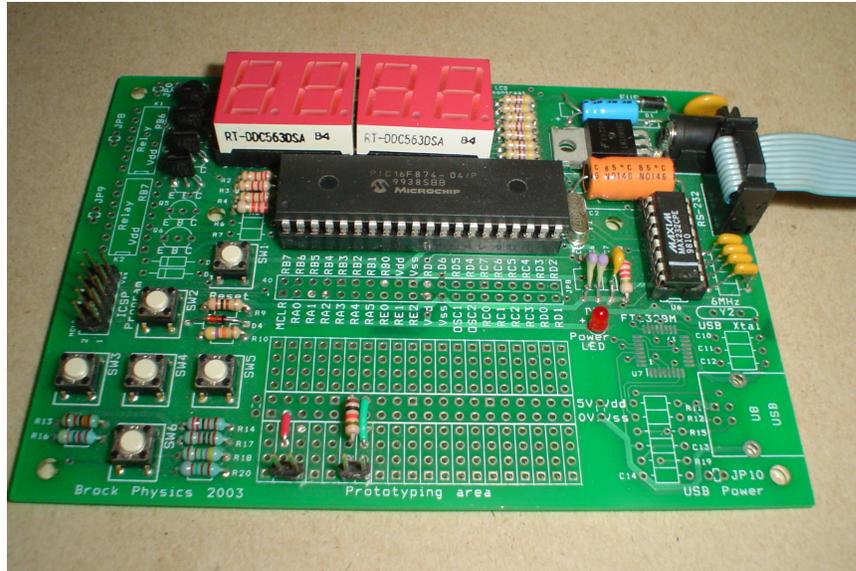
Figure 4.2: A completely assembled PICLab project board
