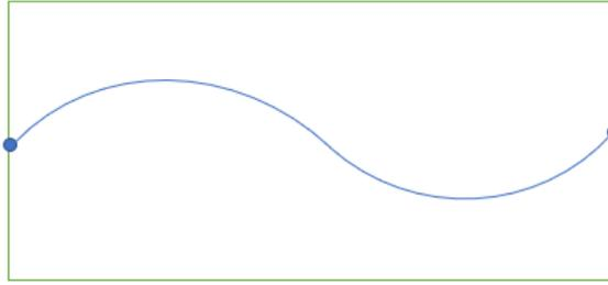
Figure 2: The second resonant frequency fits a whole wavelength exactly in the tube, causing  $L = \lambda$ .
