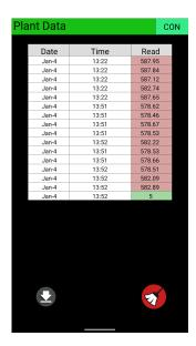
BT connection is done through MAC address (status in top right). It also has options to connect to a specific device name ("HC-05") if needed.
